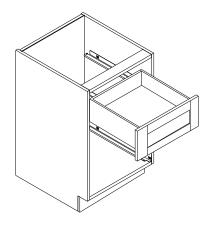
**Step 5:** After that, a small lever on the drawer front connector can be used to make small adjustments to correct clearance. Check the stability of the cabinet and make adjustments by tightening the cam locks.
