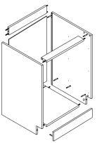
**Step 2:** Attach the Undermount soft-close slides onto the side panels using the pre-drilled holes and the nickel round head screws.
