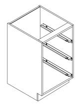
**Step 3:** Assemble the drawers and install the drawer front connector on the underside of the bottom panels of the drawers, secure with short screws.
